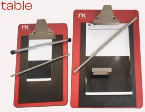
Designed to draw down sample coatings on test charts with a high degree of reproducibility.
