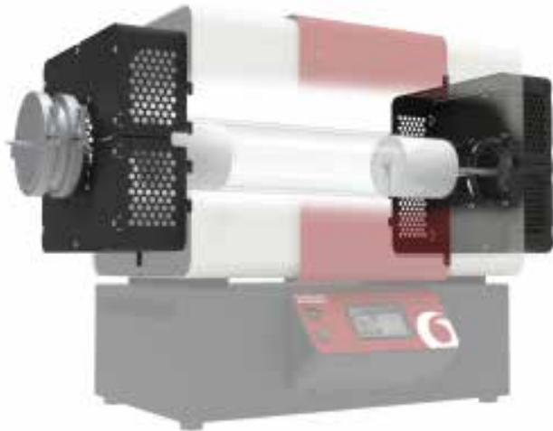
Work tube packages with extended length work tubes include guards as indicated in this image. The guards simply hook into the end plates of the tube furnaces and are each fixed with one screw.
